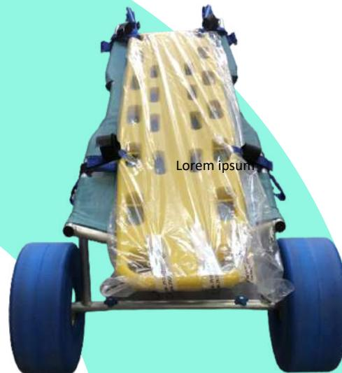
The design that it presents is a plastic floating spinal board fix to an aluminum support, which is the chassis.
